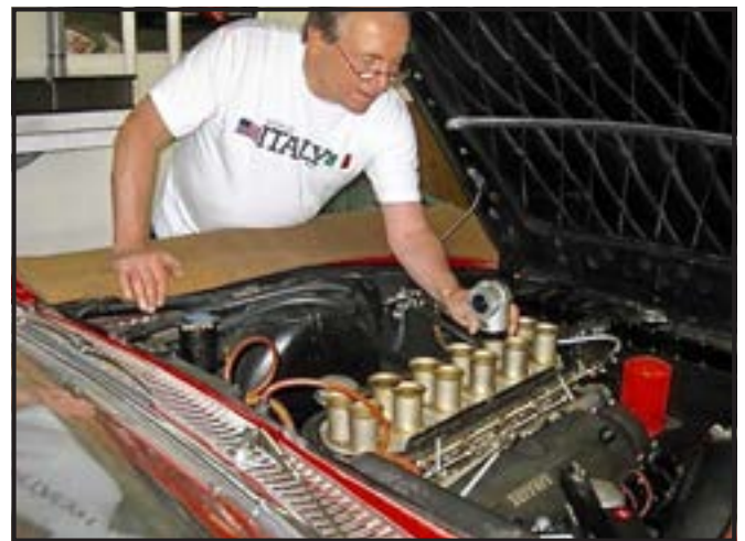
The “Official” interpreter’s son contemplates tuning six Weber carburetors all at once.
