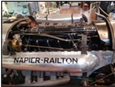
The 580-hp W12 (three 4-cylinder banks) up close
