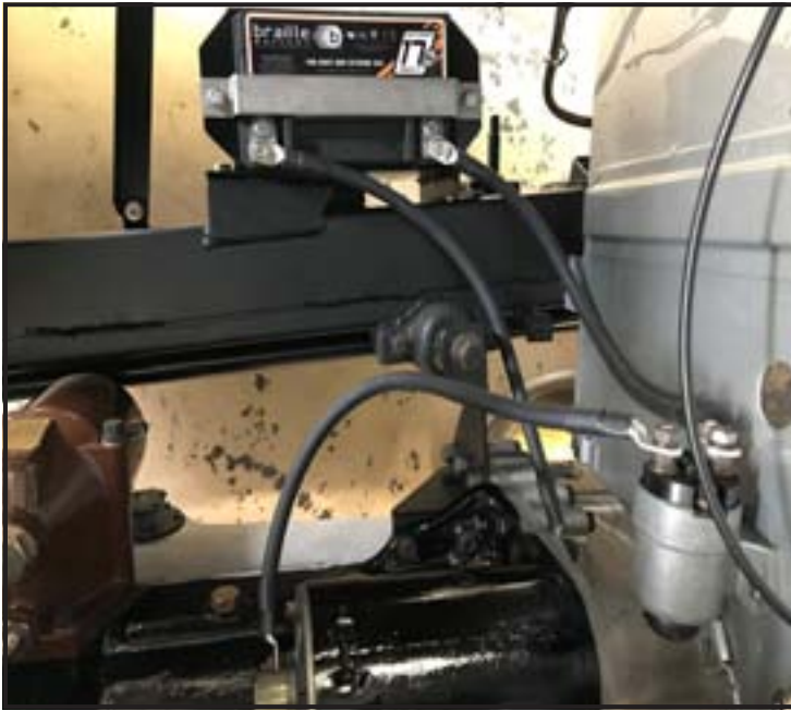
Top view of battery box, mounted on existing RHD M/C bracket.
