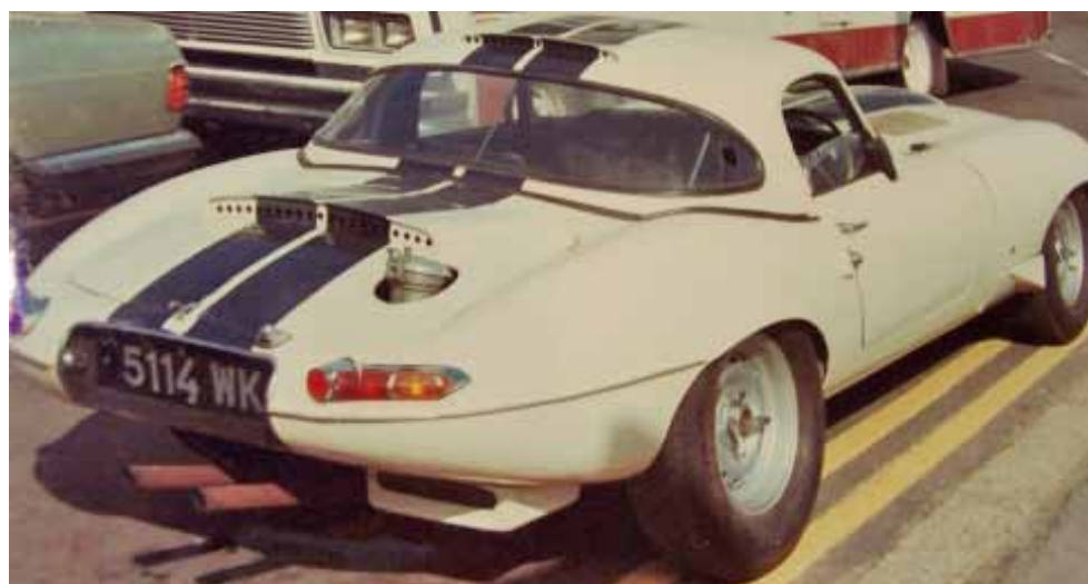
Bill's Lightweight after restoration. Note the oil radiator on the underside and the triangular piece required by Le Mans rules to cover enough of the perimeter of the wheel.
