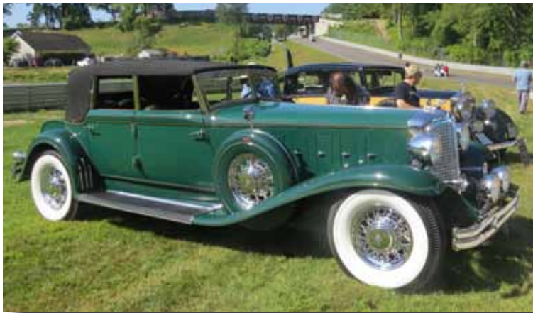
This '32 Imperial had its body and interior crafted by LeBaron. Buyers of high-end cars in the 1920s and 1930s often bought an engine and chassis from a car company and had an independent body and interior company complete a custom made product.
