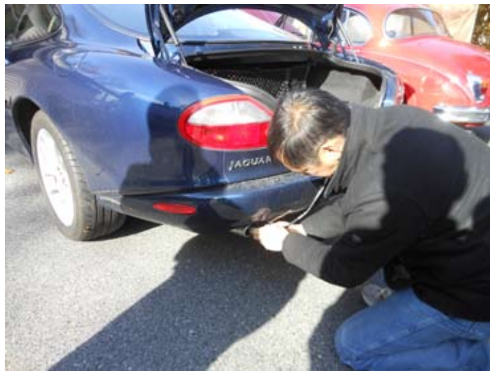
Left: John Feng inside Carl Hanson's XKR holding a stoichiometer with a reading of 15. The meter is connected to the tailpipe (right) and measures air/fuel ratios under various conditions. Good range is between 14.5 and 16. Photos courtesy Carl Hanson.
