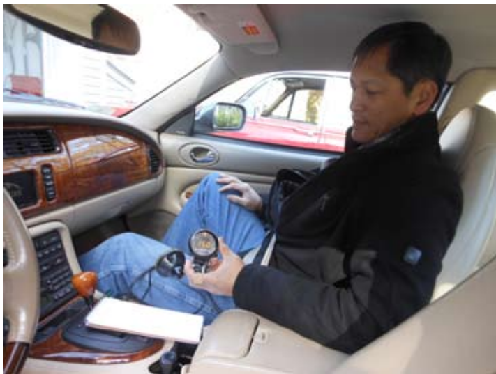
Left: John Feng inside Carl Hanson's XKR holding a stoichiometer with a reading of 15. The meter is connected to the tailpipe (right) and measures air/fuel ratios under various conditions. Good range is between 14.5 and 16. Photos courtesy Carl Hanson.
