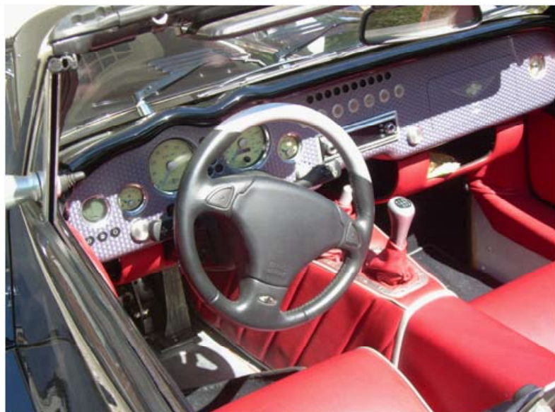
Figure 4. The Mog's tight little cockpit and machined aluminum dash with minimalist instrumentation.
