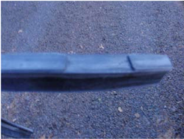
The notch in the rubber seal to accept the sill plate fastener.
