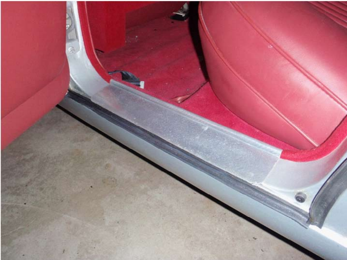
New, snug rubber door seals muffle road noise, prevent moisture from entering and really improve the look of the threshold.
