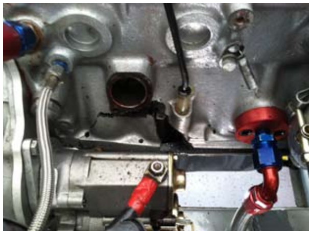
Catastrophic failure! The side of the Sprite motor (left) shows a hole where the connecting rod tried to exit. Viewed from the top, a cylinder left vacant by the disintegrated piston.
