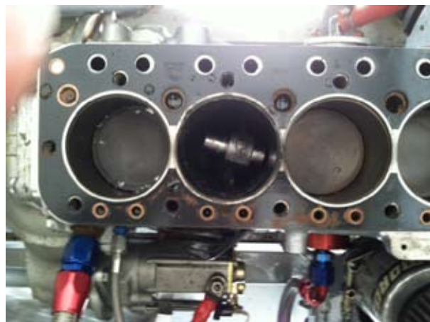
Catastrophic failure! The side of the Sprite motor (left) shows a hole where the connecting rod tried to exit. Viewed from the top, a cylinder left vacant by the disintegrated piston.
