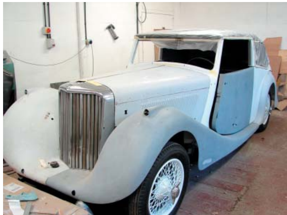
The MK IV as received at Davenport Cars, with doors, hood, and grille parts being aligned
