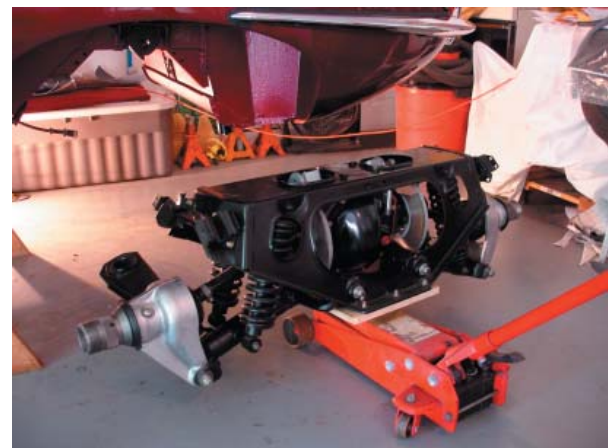
The moment of truth - George's IRS ready to be lifted up into the car
