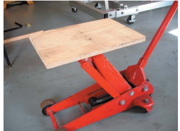
Note the countersunk holes in the plywood to accommodate the flat-head bolts
