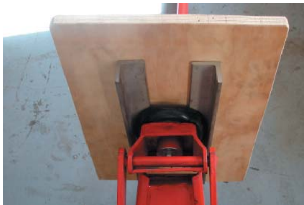
The view from below, showing the angle stock supporting the plywood, all securely bolted to the jack's pad
