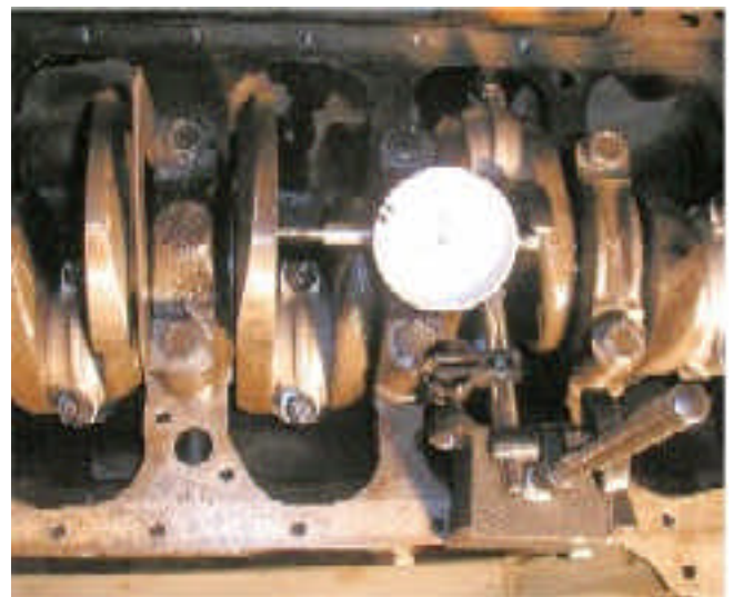
Figure 2 Checking for crankshaft end float
