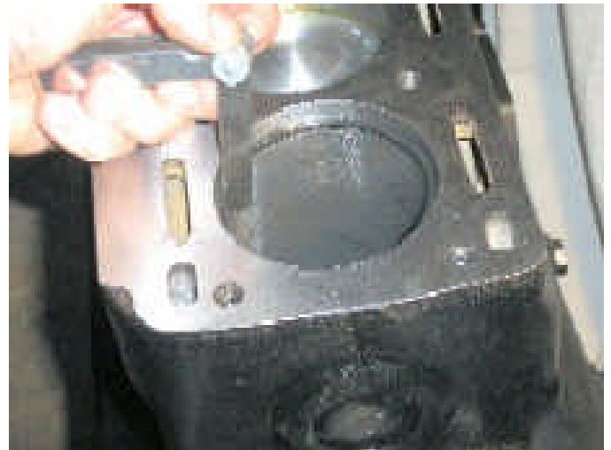
Figure 4 Checking ring end gap
