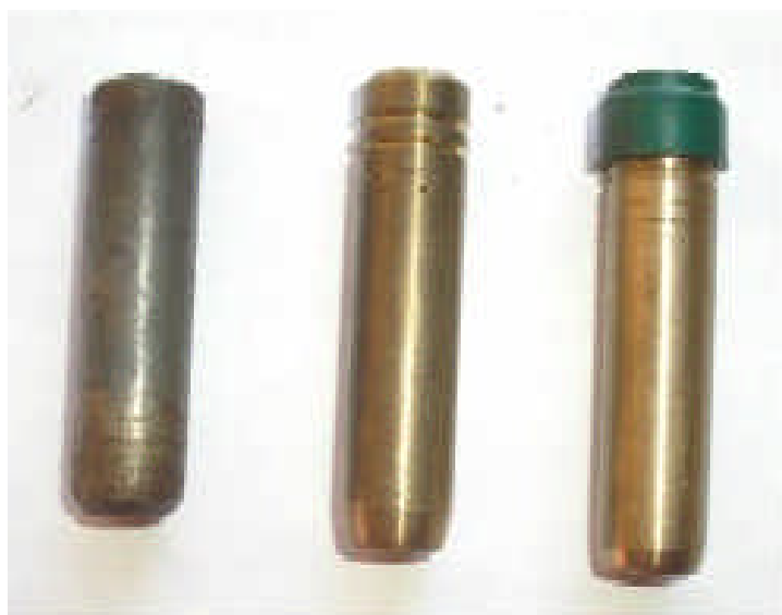
Figure 1 Valve guides, old new and with seals installed
