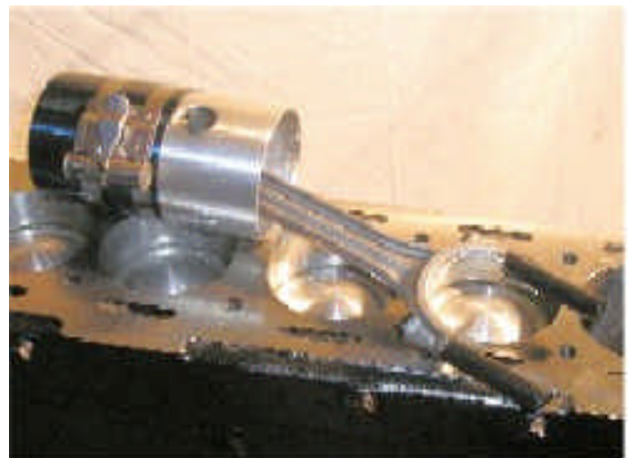
Figure 5 Piston ring compressor with rubber protecting rod bolts
