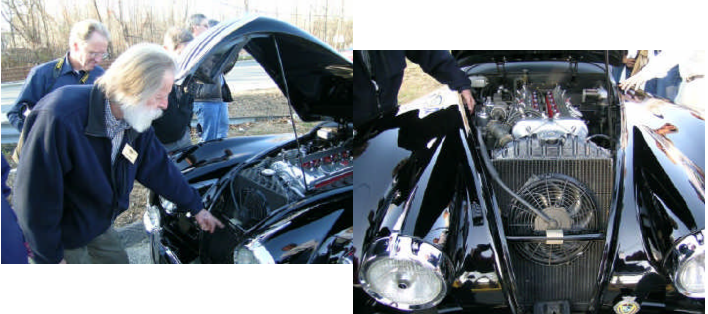
Left: Paul Rikert shows of his auxiliary cooling system, FANTastic". Right: A really neat installation, removable for Concours competition
