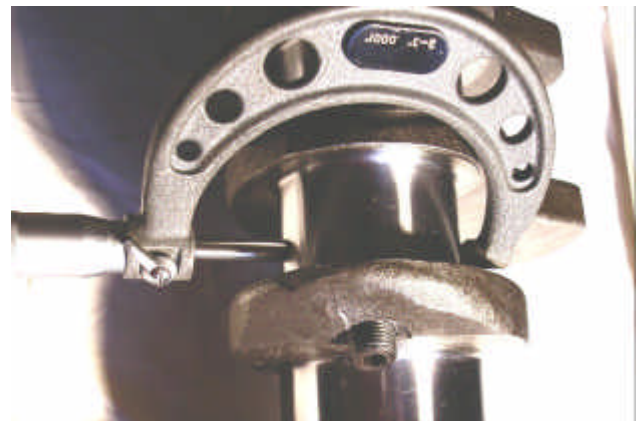
Above Measuring the crankshaft with a micrometer
