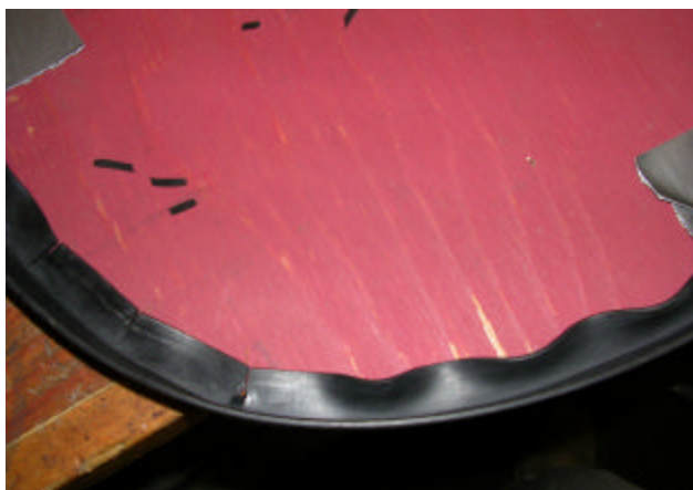
Figure 5 Gasket Puckering At The Corners
