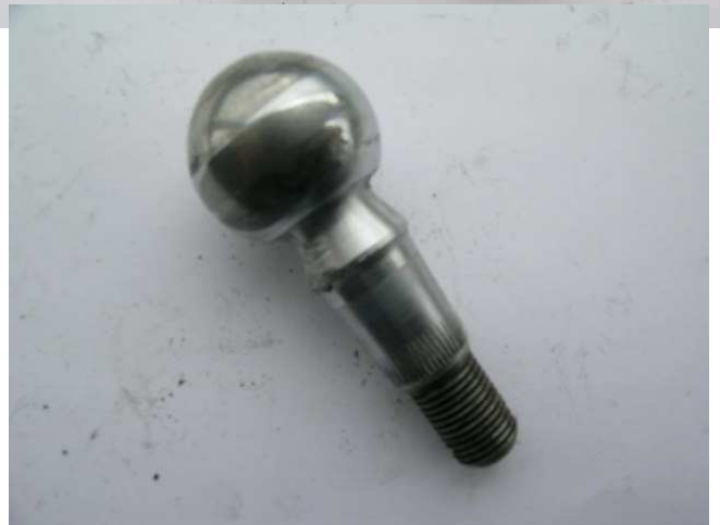
Above: Worm out lower ball joint. Wear is on the top which carries the weight of the MK IX
