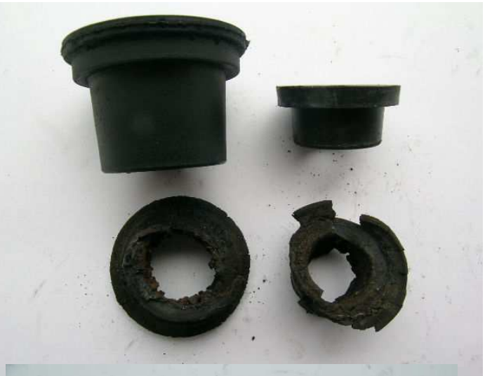
Above: The MK IX in Adrian Curtis's garage Below: The new bushings on top and the worn out originals below
