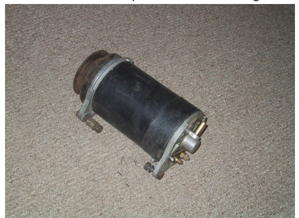
Early generator with oiler for the rear bronze bush
