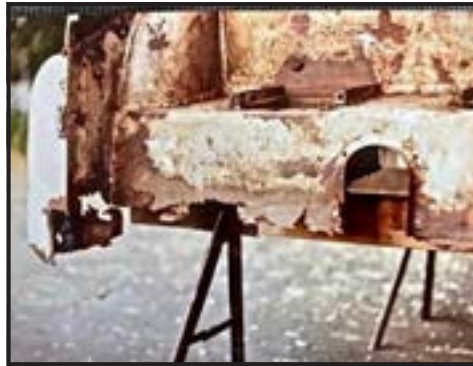
Original rusted out battery box shelf
