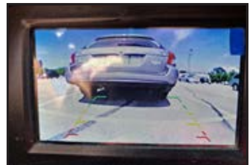
Here's the monitor display in a typical parking lot situation. Note the backup lines. Nice!
