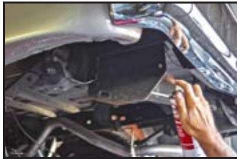
Here a spray can directly covers the surfaces behind the area bumper.
