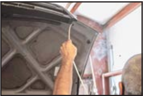
And now we protect cavities in the hood, er, bonnet.
