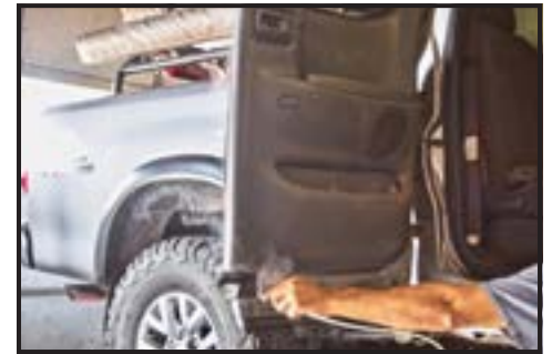
Now we get the door cavities protected.
