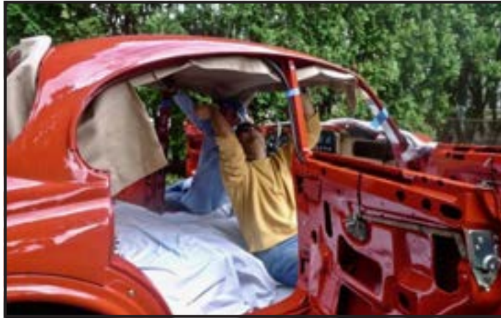
Carl Hanson and Eric Kriss helping with the challenging job of installing the headliner on its bows.
