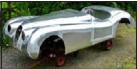
XK120-LT Magnesium Bodies created in case new XK120-Cs were not ready in time for LeMans 1951 ( https://www.bonhams.com/auctions/17259/lot/53/ )
