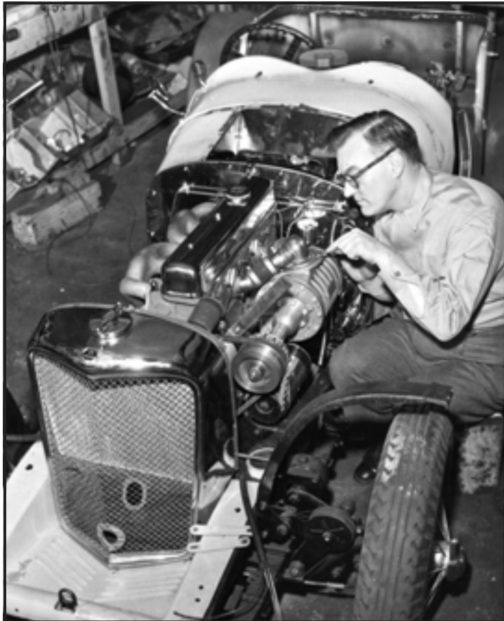
Dave hard at work on the supercharger he added to the original SS100 engine
