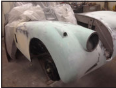
New sheet metal has been added . . .
