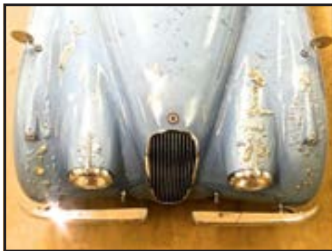
George's XK-120's front end suffered from blistering paint due to the heat of the fire it was exposed to.
